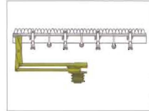
One-sided drive for rocker arm and connecting rods for front bars.
